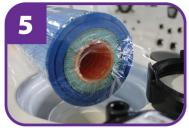
Remove filter and take it out of the plastic transport bag. Leave filter canister open when filling.
